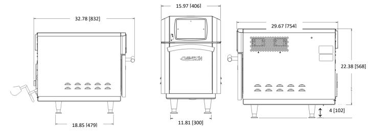
Measurement Units: Inches [Millimeters]
